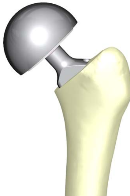
Figure 10: Implanted bipolar head
